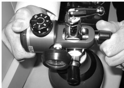
**FIGURE 3.1** Attaching the IOCI00P to the Cylinder
